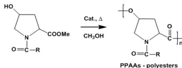
**Figure 3:** Synthesis of the PPAAs-PEs by thermal polycondensation of N-substituted *trans*-4-hydroxy-proline methyl ester.
