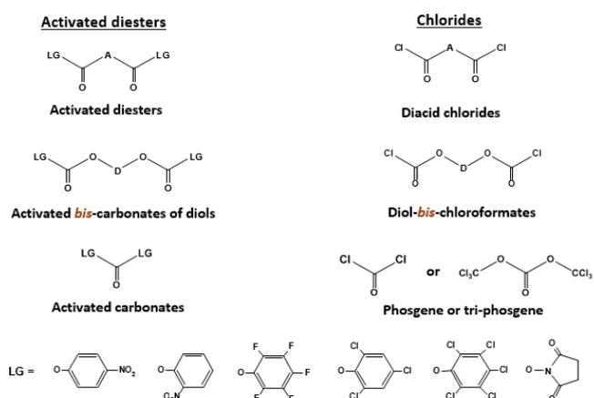
**Figure 10:** Some key *bis*-electrophilic monomers for synthesizing PPs. A – a diacid residue, D – a diols residue.
