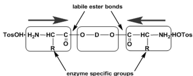
**Figure 9:** The structure of DADEs – key monomers for synthesizing PPs.
