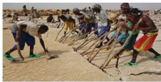
Figure 4: levering up slabs of layered salt crust
