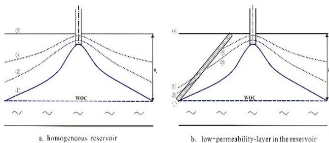
Figure 2: Reservoir bottom water coning diagram.
